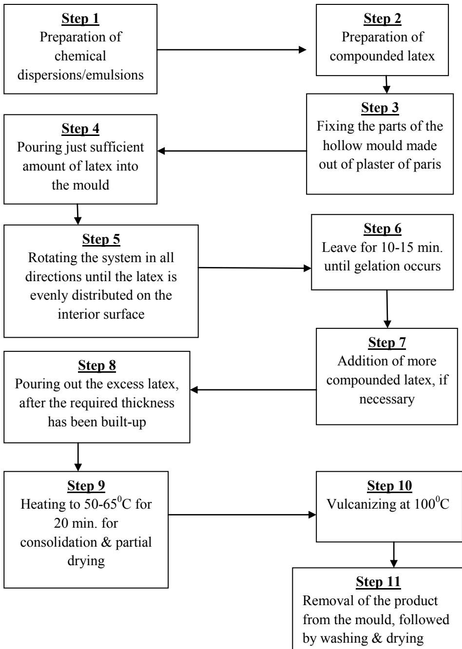
The complete manufacturing procedure giving each of the steps involved in the production of a casting using plaster of paris moulds according to the rotational moulding technique is shown in the above flow diagram.
