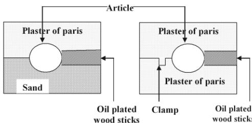
Schematic diagrams showing the preparation of a two piece plaster of paris mould
