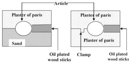
Schematic diagrams showing the preparation of a two piece plaster of paris mould
